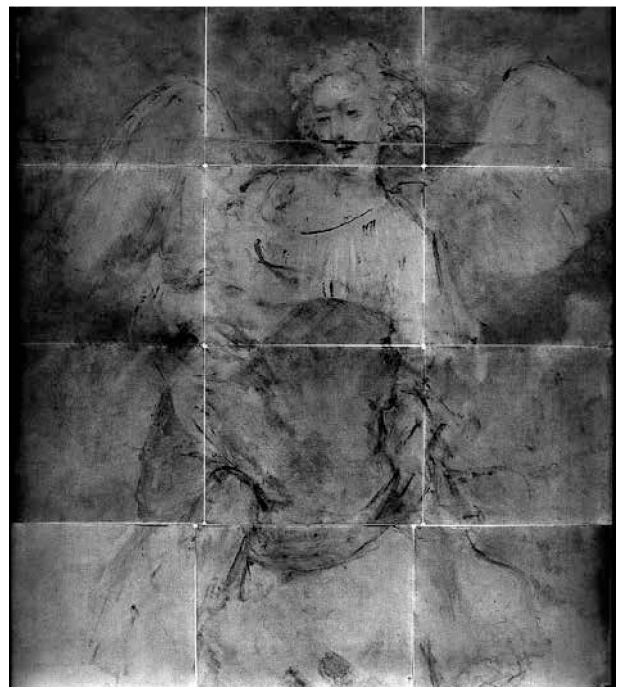
Fig. 11 4 th autoradiograph, film exposure 7 d-51 d after the end of activation, contributing isotopes 76 As, 32 P, 60 Co, 203 Hg. – (Autoradiograph C. Laurenze-Landsberg / W. Leuther).
