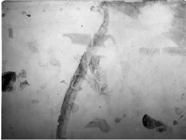
Fig. 36 4 th autoradiograph, film exposure 8 d-14 d after the end of activation, contributing isotopes ^{32}\text{P} , ^{60}\text{Co} , ^{203}\text{Hg} . – (Autoradiograph W. Leuther).
