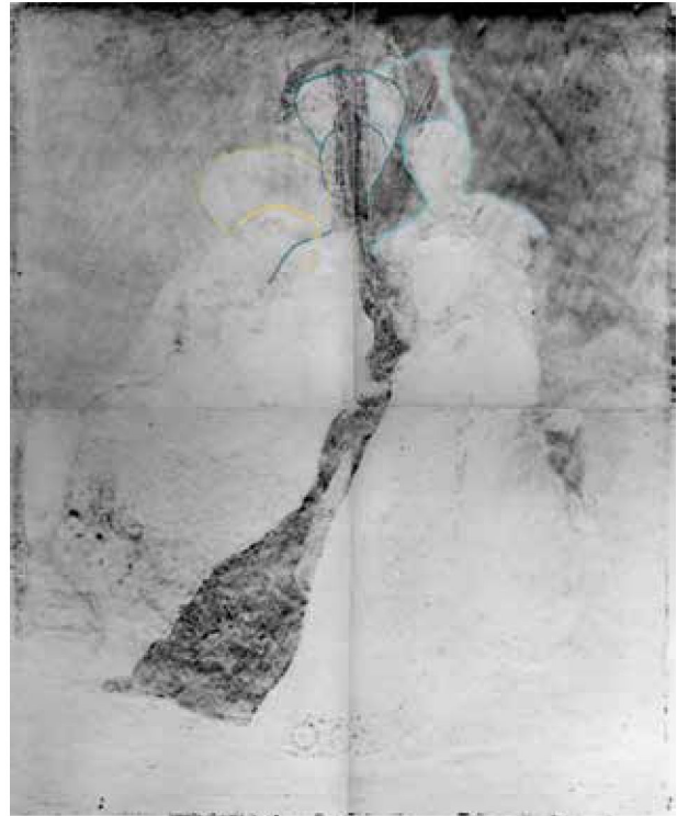
Fig. 22 4 th autoradiograph, film exposure 1 d 7 hrs-3 d 3 hrs after the end of activation, contributing isotopes 64 Cu, 76 As. – (Autoradiograph C. Laurenze-Landsberg / W. Leuther; markings C. Laurenze-Landsberg).
