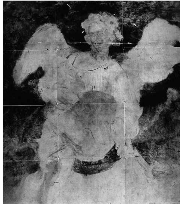
Fig. 10 2 nd autoradiograph, film exposure 12 hrs 30 min-3 d after the end of activation, contributing isotopes 56 Mn, 64 Cu, 76 As. – (Autoradiograph C. Laurenze-Landsberg / W. Leuther).
