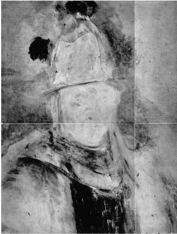
Fig. 3 3 rd autoradiograph, film exposure 1d-4d after the end of activation, contributing isotopes ^{64}\text{Cu} , ^{76}\text{As} . – (Autoradiograph C. Laurenze-Landsberg / W. Leuther).
