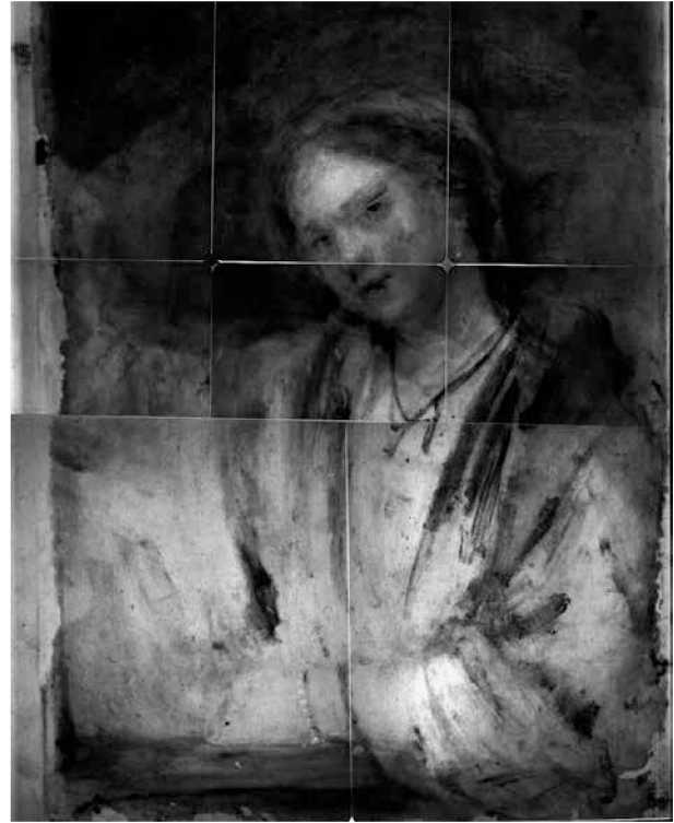
Fig. 8 6 th autoradiograph, film exposure 13 d-27 d after the end of activation, contributing isotopes 32 P, 60 Co, 203 Hg. – (Autoradiograph C. Laurenze-Landsberg / W. Leather).
