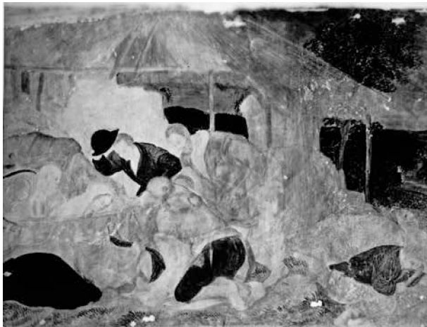
Fig. 29 1 st autoradiograph, film exposure 30min-3 hrs after the end of activation, contributing isotopes ^{56}\text{Mn} , ^{64}\text{Cu} , ^{76}\text{As} . – (Autoradiograph W. Leuther).
