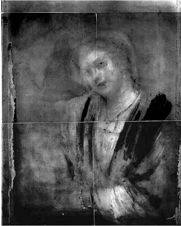
Fig. 7 3 rd autoradiograph, film exposure 1 d 4 hrs-3 d 10 hrs after the end of activation, contributing isotopes 64 Cu, 76 As. – (Autoradiograph C. Laurenze-Landsberg / W. Leather).
