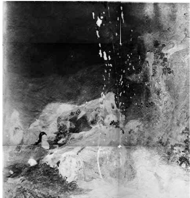
Fig. 18 2 nd autoradiograph, film exposure 25 hrs-50 hrs after the end of activation, contributing isotopes 64 Cu, 76 As, 24 Na. – (Autoradiograph C. Laurenze-Landsberg / W. Leuther).
