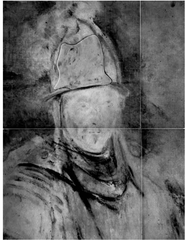
Fig. 4 5 th autoradiograph, film exposure 11d-23d after the end of activation, contributing isotopes ^{32}\text{P} , ^{60}\text{Co} . – (Autoradiograph C. Laurenze-Landsberg / W. Leuther).
