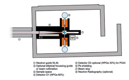
Fig. 5 Floor view of the PGAA instrument with the exchangeable units for PGAI and neutron imaging.  $-(\bigcirc$  by the authors).
