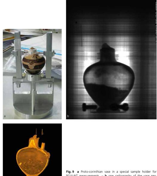
**Fig. 9 a** Proto-corinthian vase in a special sample holder for PGAI-NT measurements. – **b** one radiography of the vase performed at the PGAA instrument: the lower tightening. Screws are made of PE, upper holders from FTPE. – **c** reconstructed 3D neutron tomography image shows powder inside. – (© by the authors).
