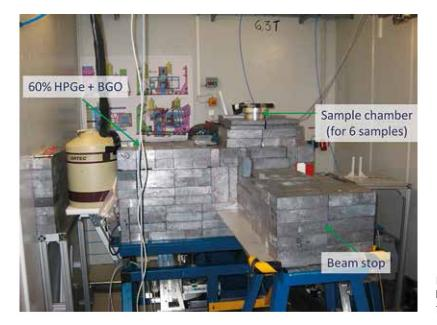
**Fig. 3** PGAA instrument in a concrete bunker heavily shielded by lead to minimize the background signal. – (© by the authors).
