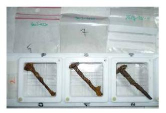
**Fig. 8** Roman nails from  $2^{nd}-3^{rd}$  century excavated in Güglingen, Germany, analysed for the chlorine content before desalination treatment. – (© by the authors).
