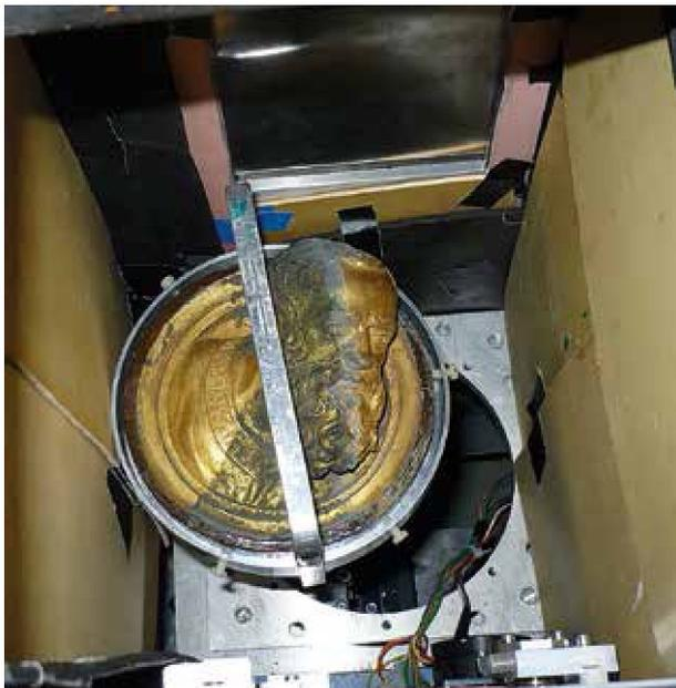
**Fig. 11** Bronze relief by Lorenzo Ghiberti in a sample holder for tangential irradiation for PGAA. – (© by the authors).
