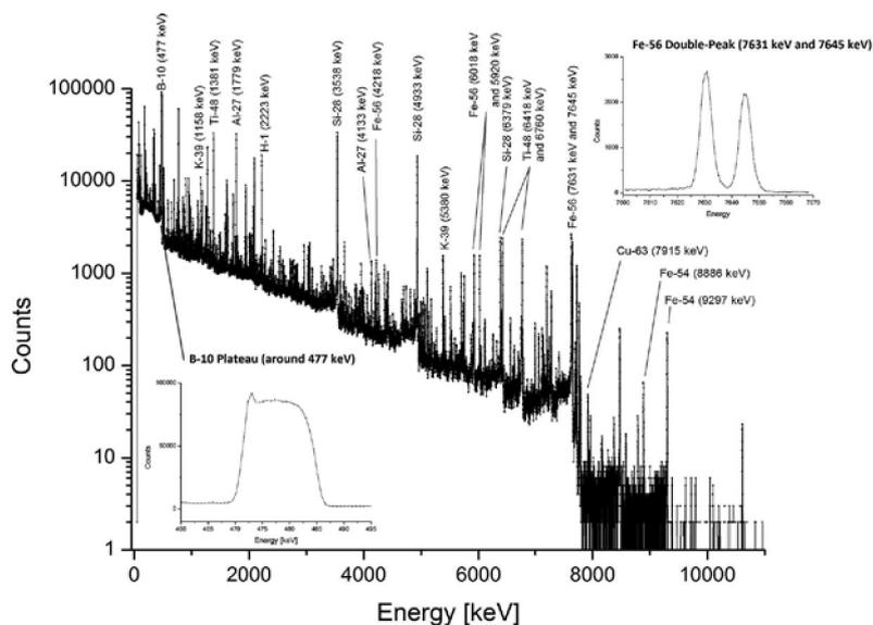
**Fig. 6** A typical PGAA spectrum. Here an example of one clay crucible sample presented in fig. 4. – (© by the authors).
