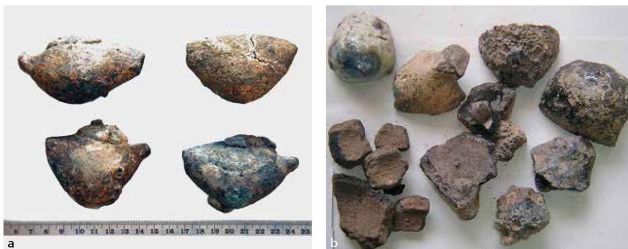
**Fig. 7** **a** intact clay crucibles found near Preslav, Bulgaria. – **b** some broken clay crucible pieces from Nadarevo near Preslav were homogenized and measured with the PGAA technique. – (© by the authors).
