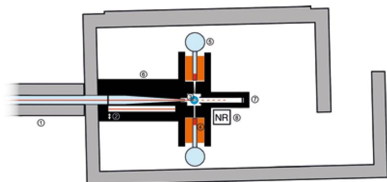
**Fig. 5** Floor view of the PGAA instrument with the exchangeable units for PGAI and neutron imaging. – (© by the authors).
