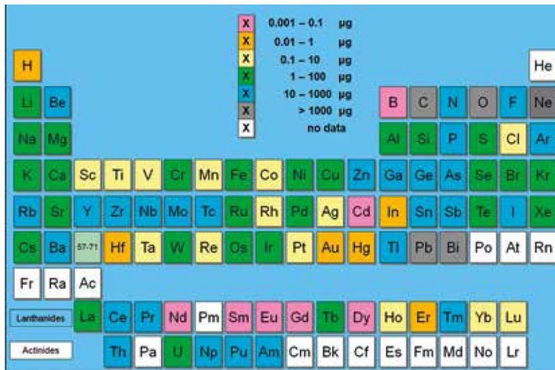
**Fig. 2** Overview of elements detectable with PGAA and expected detection limit range. – (© by the authors).
