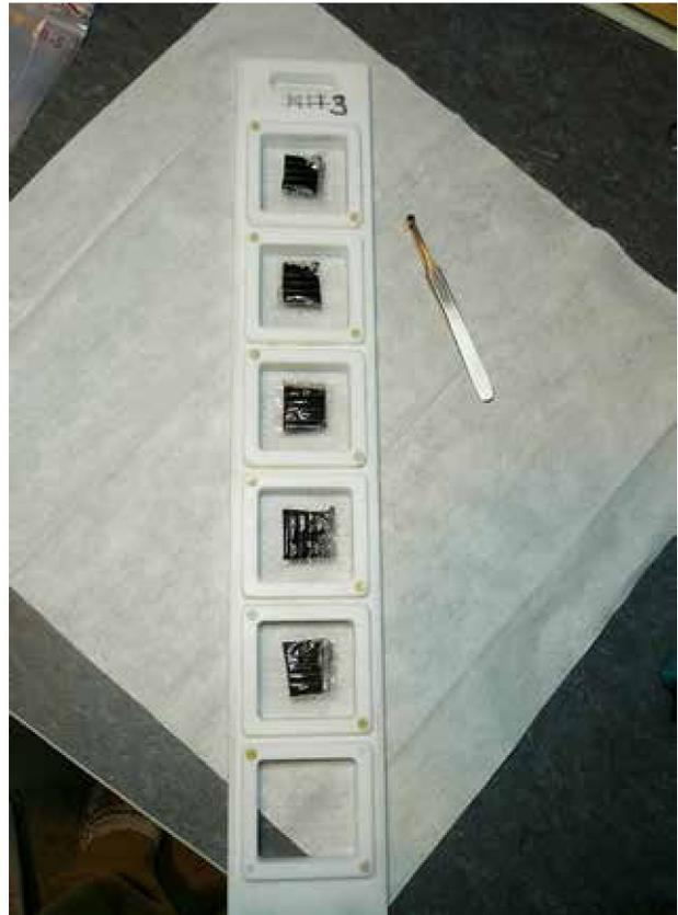
**Fig. 4** PGAA sample ladder made of FTPE can accommodate up to six samples measured automatically in one batch in possibly evacuated sample chamber. Five homogenized clay crucible samples (see fig. 7) are sealed in FTPE foil here. – (© by the authors).
