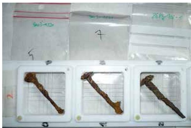
**Fig. 8** Roman nails from 2<sup>nd</sup>-3<sup>rd</sup> century excavated in Göglingen, Germany, analysed for the chlorine content before desalination treatment. – (© by the authors).
