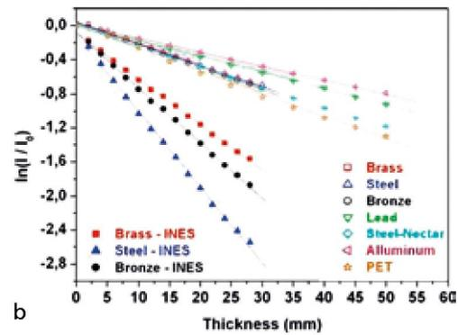
**Fig. 2** a bronze, steel and brass step wedges. – b relative beam intensity as a function of the step thickness obtained at INES with the imaging system composed by the MANTAG-032B camera and thermal neutron screen NDG 450 mm thick scintillator and obtained at NECTAR with the ZnS(Ag) pp matrix scintillator 2 mm thick. – (Graphic/photo by the authors).
