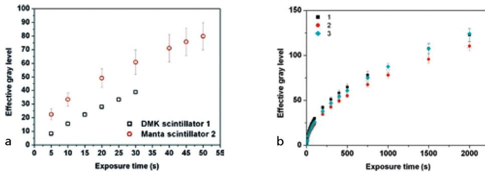
**Fig. 1** Number of effective grey levels as a function of the signal integration time for different combinations CCD-scintillator. – **a** results of INES (1 = Thermal neutron screen NDG 250 mm; 2 = Thermal neutron screen NDG 450 mm). – **b** results obtained at NECTAR (1 = ZnS(Ag) pp matrix thickness 2 mm; 2 = plastic scintillator EJ200; 3 = plastic scintillator EJ212). – (Graphic by the authors).
