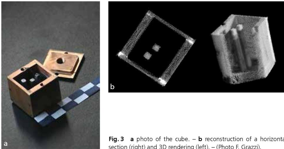
**Fig. 3** a photo of the cube. – b reconstruction of a horizontal section (right) and 3D rendering (left). – (Photo F. Grazzi).
