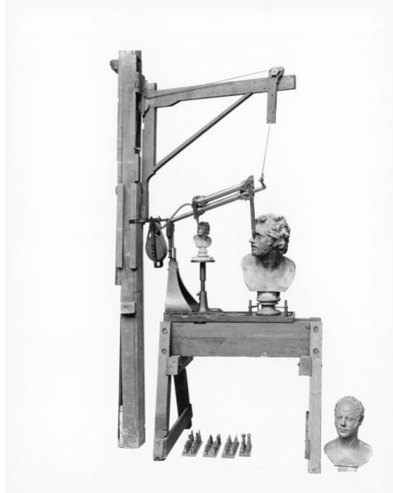
1 Benjamin Cheverton, Machine for reproducing sculpture, 1826 or 1828, cast iron, oak, plaster and wrought iron, 245 × 150 × 74 cm. Science Museum Group Collection, London, no. 1924-292 (photo © The Board of Trustees of the Science Museum, London)
