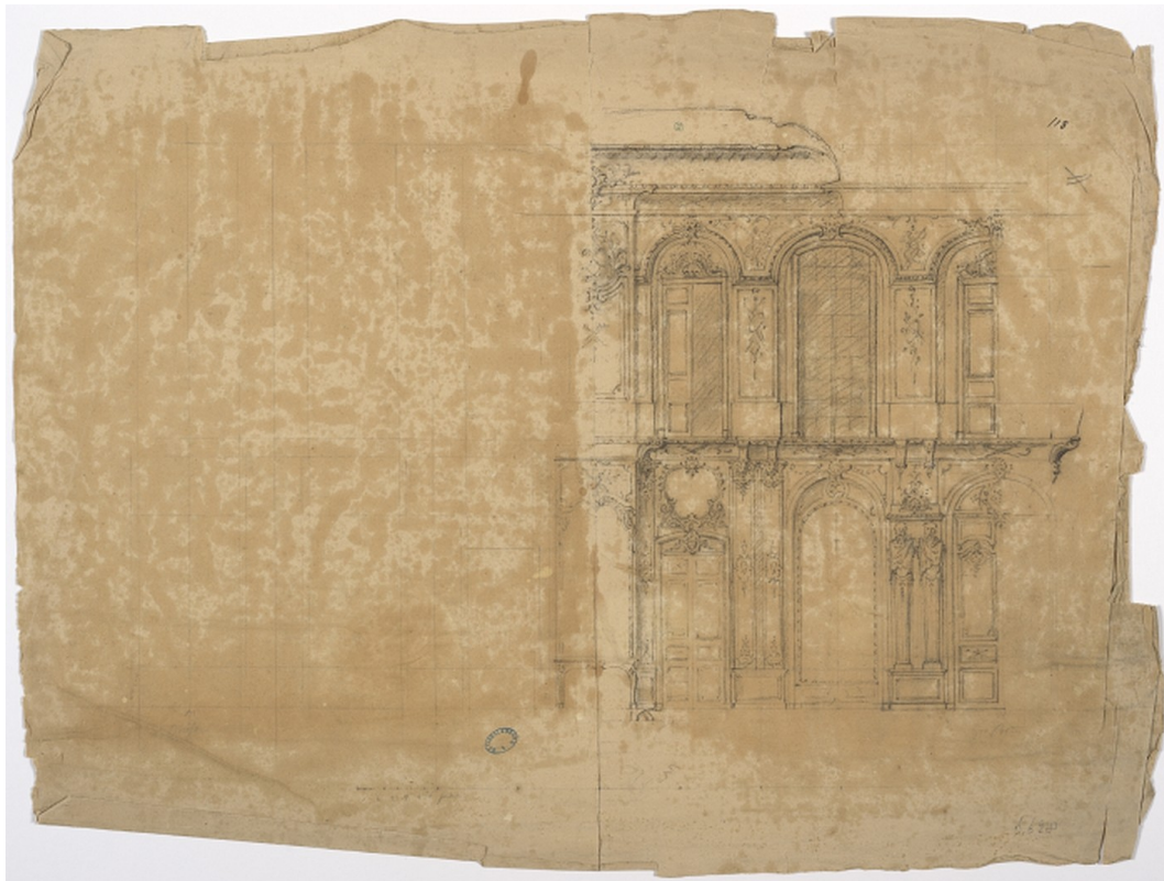
15 Anonymous French early 18th-century draughtsman, Partial elevation of a two-storey panelled interior with two doors . The oil stains on the sheet were likely caused by contact with a sheet of tracing paper that was not completely dry. Squared in graphite, black chalk on laid paper, 440 × 585 mm. Nationalmuseum, Stockholm, NMH THC 6628 (photo: Cecilia Heisser / Nationalmuseum)
