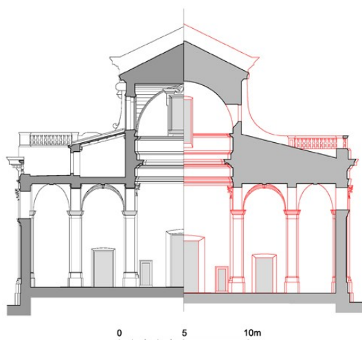
12 The Cathedral, Dubrovnik, Napoli's changes to Bufalini's design, transverse cross-section with a view towards the main façade, completed state (left), reconstructed original design (right) (architectural drawing: I. Tenšek, I. Valjato-Vrus)
