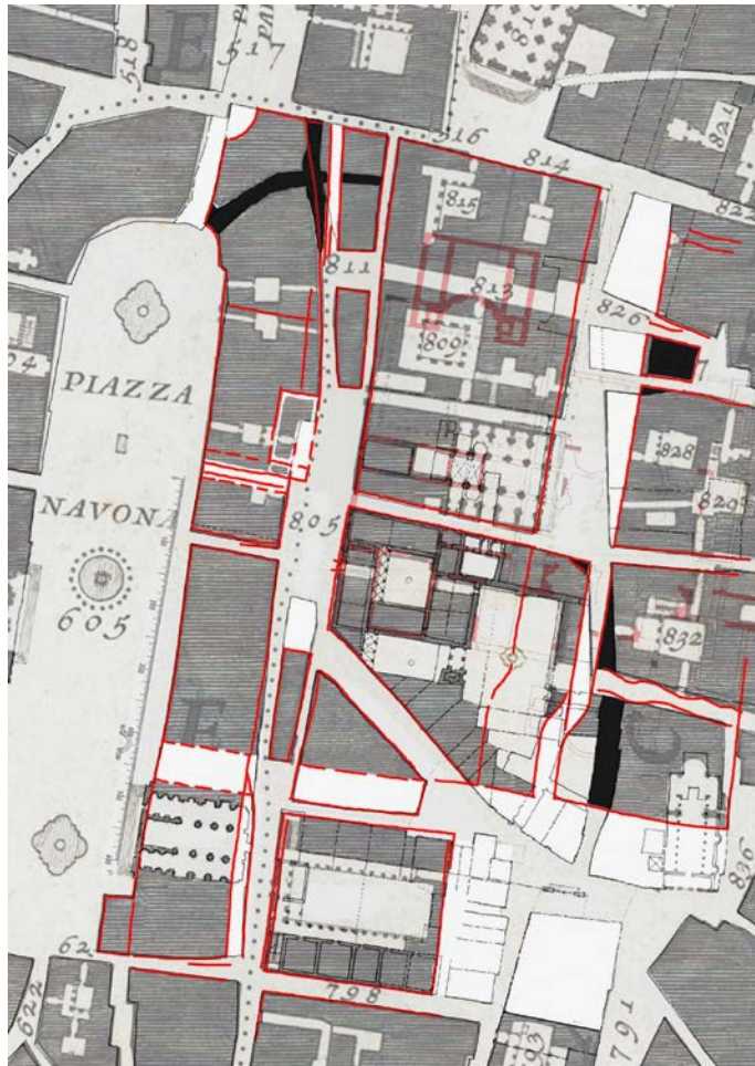
20 Antonio da Sangallo the Younger, site sketch U 1259Ar redrawn to scale, with areas of “cut” (white) and “fill” (black).
